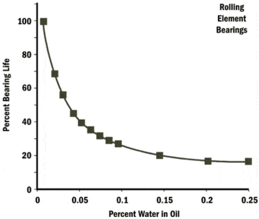
**Figure 2. Water Contamination**
